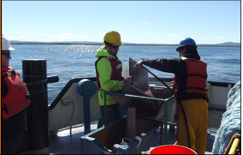
Erik Hartnett pouring a benthic sample into the elutriator aboard the R/V Lake Guardian to remove excess sediment. Credit: Sebastian Paczuski
