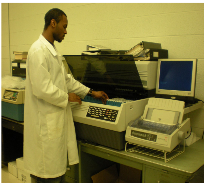
Graduate student Jaquan Williams operating Scintillation counter for measuring radioactivity in research sample.
